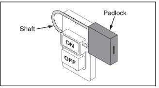
Figure 28. Switch disabling padlock inserted into ON button.
